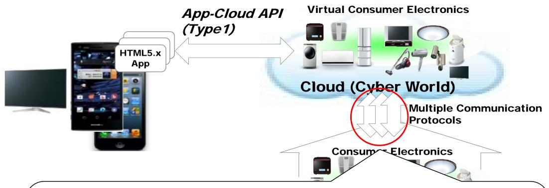
Physical CE Control Protocols such as Echonet Lite, EE-Bus, IR Control and so on are independent from Type 1 APP-Cloud API.
