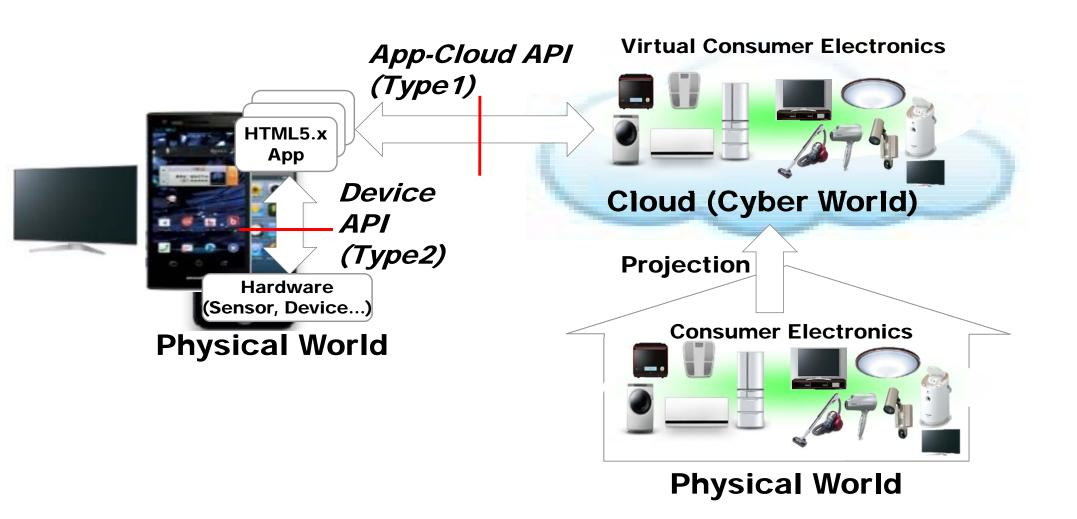
IoT could assume both App-Cloud API(Type1) and Device API(Type2) as its API to access physical Sensors, Devices and Sets such as CEs.
