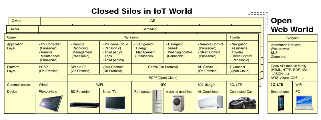
Even in 1 company, platform is easy to be designed and updated respectively according to a variety of different "Things" characteristics.
