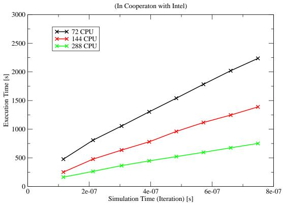
Intel Xeon Processor: X5650 B0; Frequency: 2.93 GHz # processors 2; # cores 6; Cache (L1 KB/L2 MB/L3 MB): 32 KB / 256 KB / 12 MB; 6x4GB DDR3 1333 RDIMM QDR InfiniBand 4x
