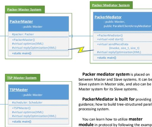
**Packer mediator system** is placed on between Master and Slave systems. It can be a Slave system in Master side, and also can be a Master system for its Slave systems.
