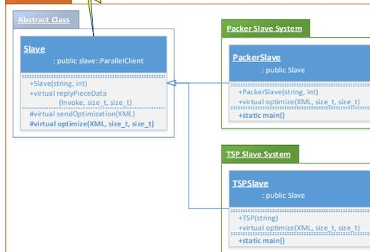
**Slave** is an abstract and example class has built for providing a guidance; how to build a Slave system belongs to a parallel processing system.
